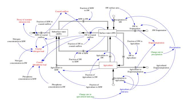
Figure 29: Stock-flow model structure for water availability for agriculture sector and its interactions with inland and coastal natural sub-systems. The main input and output variables are shown in blue and red, respectively. Change driving variables are shown in green in relation to hydro-climatic and land use changes.
