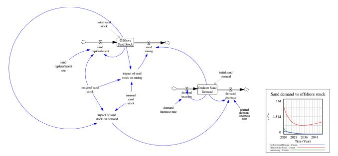
*Figure 24 Model construct for offshore sand mining with interaction of demand, resource renewal and resource use.*
