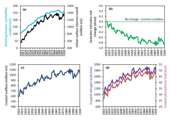
Figure 35: Demonstration results of the generic model construct for water availability for urban and tourism sector under RCP4.5 and SSP1 change scenarios in MAL3: (a) municipal water availability and urban storm water, (b) seawater intrusion risk, (c) coastal outflow, and (d) coastal nutrient loads.
