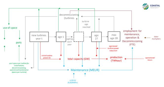
*Figure 16 Port and Energy model focusing on the logistics and economic impacts of decommissioning offshore wind turbines (see deliverable D14).*
