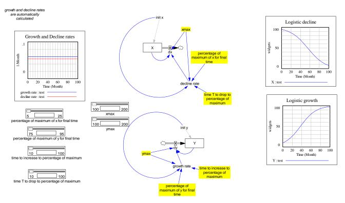
*Figure 9 Automatic calculation of growth and decline rates from target values and time to reach these.*
