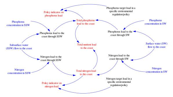
*Figure 36: Stock-flow model structure for evaluating the implementation of environmental regulations/policies on coastal water quality. The main input and output variables are shown in blue and red, respectively.*
