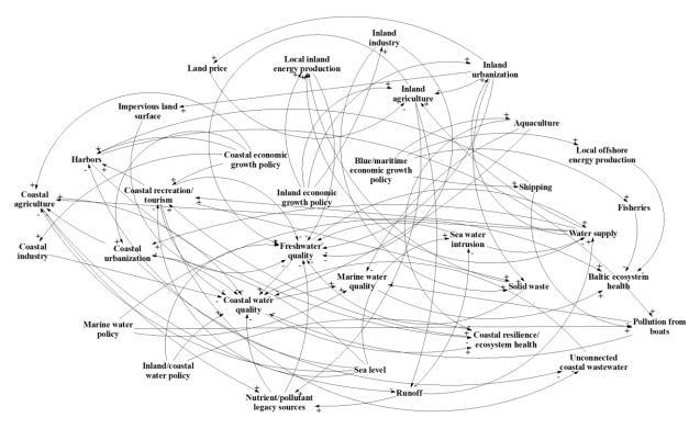
*Figure 26: Regional causal loop diagram (CLD) for MAL3. Positive (negative) interactions represent the same/reinforcing (opposite/balancing) change directions for the connecting system components.*
