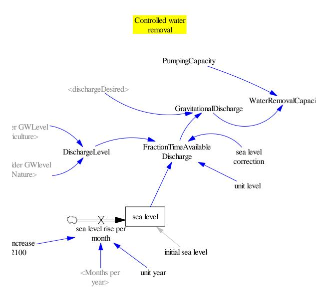
Figure 19 Model construct for the impact of sealevel rise on the operational window for discharging water to the sea as an strategy for water management.
