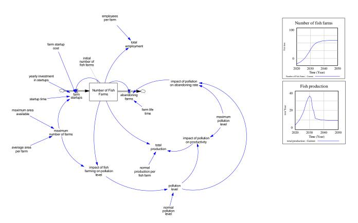
*Figure 13 Generic structure for starting up a new sector, with fish farming as an example.*
