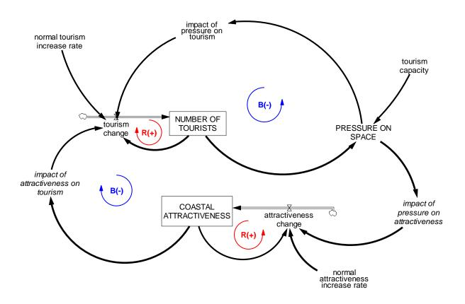
Figure 2 Tutorial example of a stock-flow model for tourism development used during the project kickoff meeting (June 2018) with reinforcing (R) and balancing (B) feedback loops indicated.
