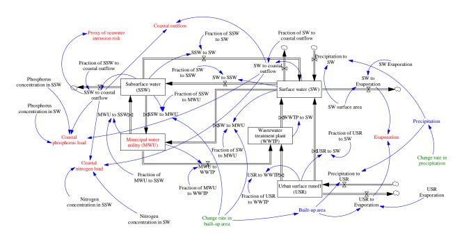
Figure 33: Stock-flow model structure for water availability for urban and tourism sector and their interactions with inland and coastal natural sub-systems. The main input and output variables are shown in blue and red, respectively. Change driving variables are shown in green in relation to hydro-climatic and land use changes.
